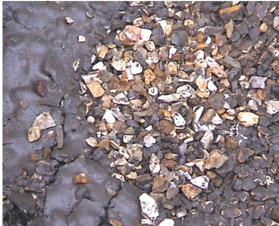
A Design A (see Figure 5), the gravel surface, showing area cleaned by one small nozzle
